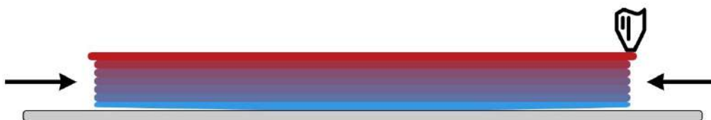
Figure 5: Print warp due to thermal gradient
